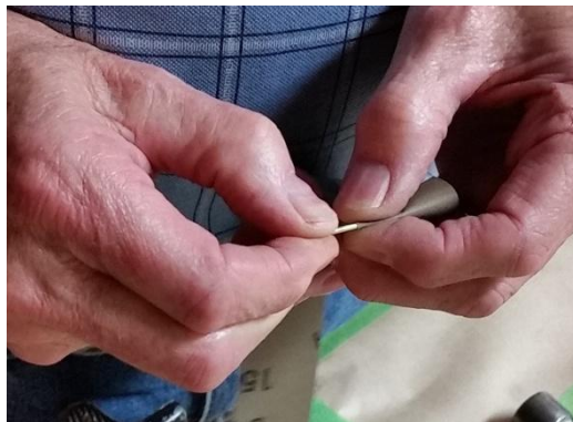
Figures 3 & 4 - Cleaning the Work and Hammering the Silver Solder Flat
